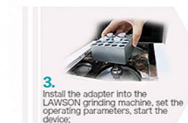
3. Install the adapter into the LAWSON grinding machine, set the operating parameters, start the device.
